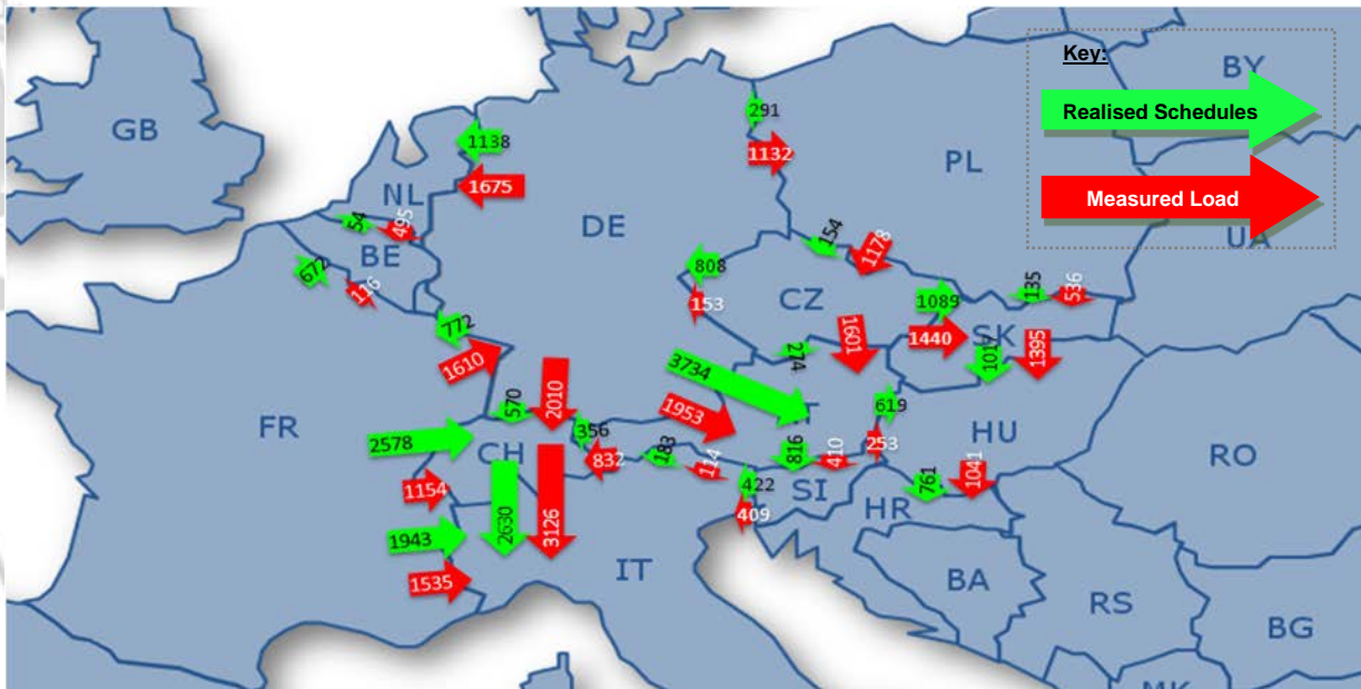
Figure 16. Average Realised Schedules and Measured Load Flow in Europe in cases when Realised Schedules DE→AT are greater than 3000 MW. Range of data: 01.2011–12.2012
