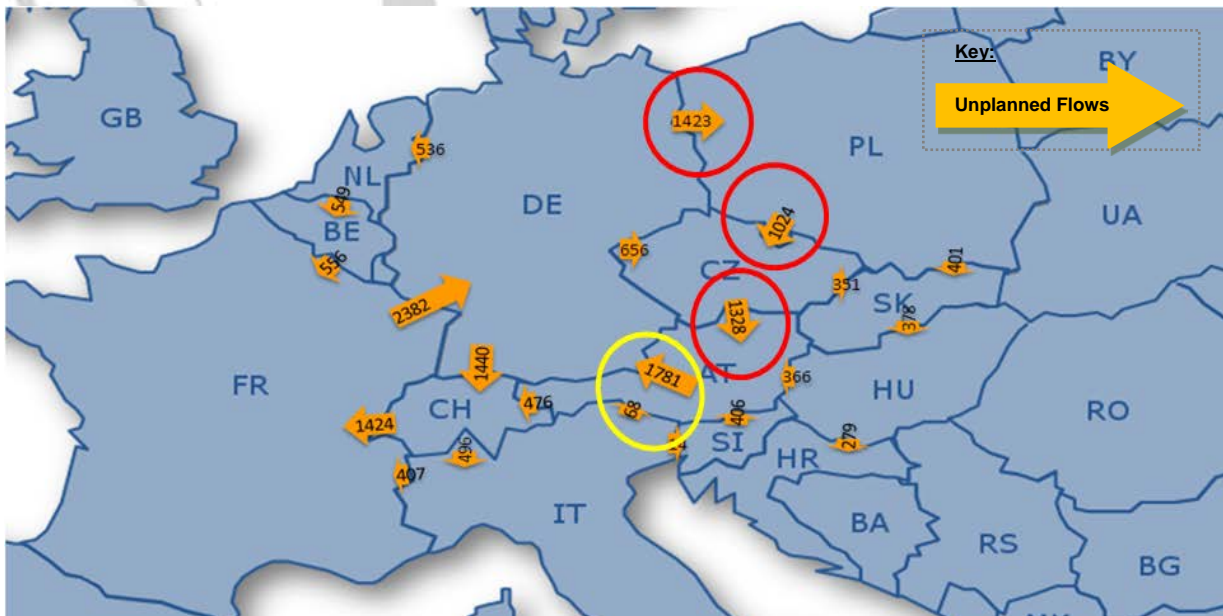
Figure 17. Average Unplanned Flows in Europe in cases when Realised Schedules DE→AT are greater than 3000 MW. Range of data: 01.2011–12.2012
